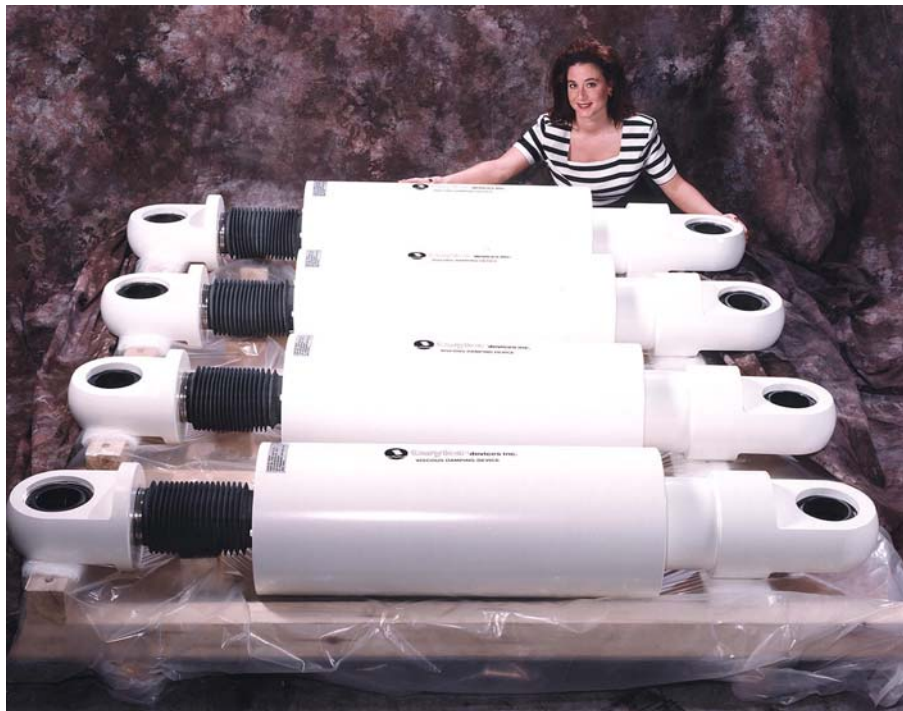
500 kip Lock-Up Devices for the Sidney Lanier Bridge (Georgia)
